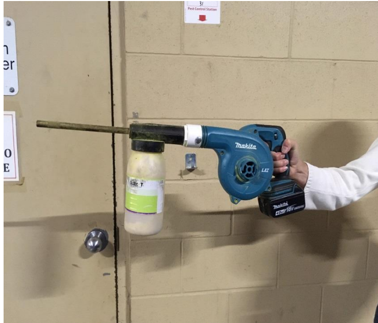
Figure 5. Makita blower used to apply Nutrimite™ © Neil Helyer, Fargo
