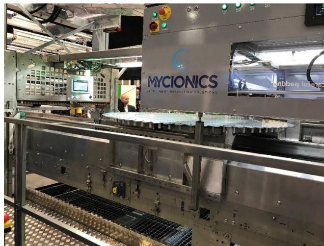
Mycionics robotic harvester for Christiaens drawer system
