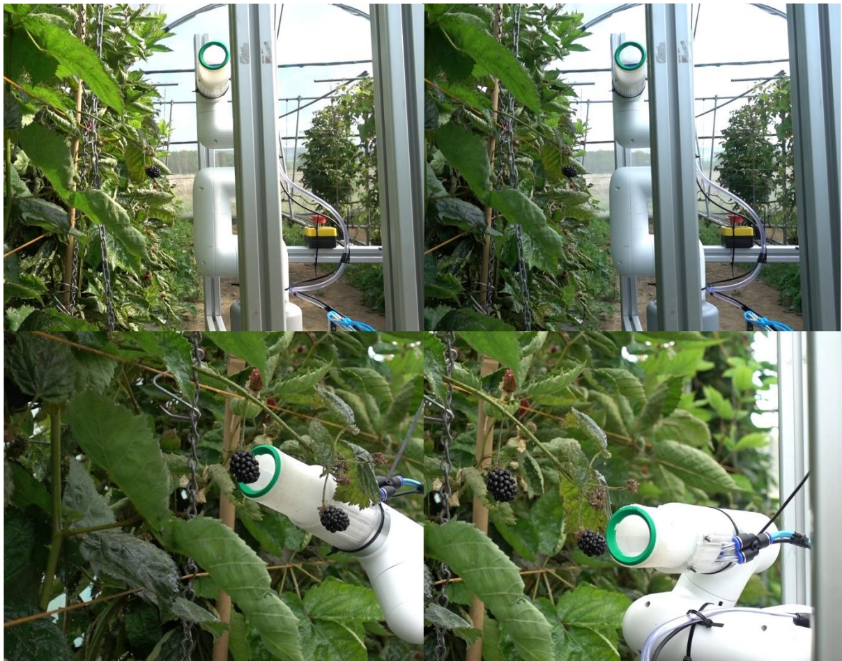
Figure 2: Top row of the image: the light variability was significant during the experiments; the two images show how the light condition changed dramatically from one moment to the next one. Below, it can be seen on two berries how the robot aligned with the wrong axis of the berry, due to the lack of a clearly elongated shape.
