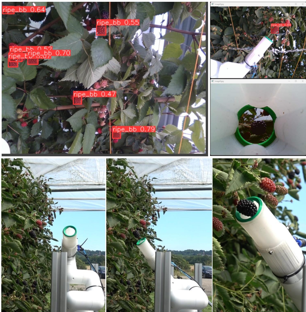
Figure 3: The improved vision algorithm detected correctly most of the berries (top left image), but the berry was still not detected with the internal camera (top row, right-bottom image). Although the algorithm aligned correctly the gripper with the berry (bottom row, central image) during the ingestion stage even small discrepancies prevented the ingestion (bottom row, right image).
