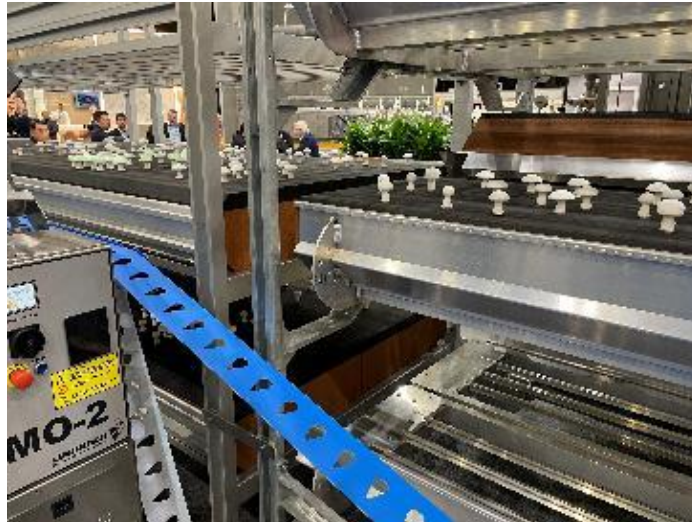
Tilting shelf growing system and moving belt from GTL
