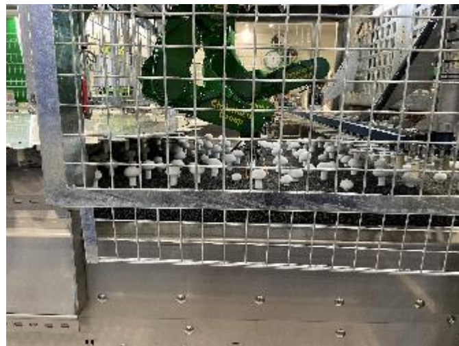
Robotic mushroom harvester from Mycionics
